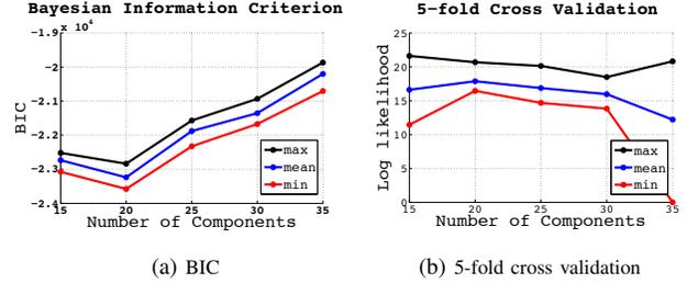
Fig. 3: The *Bayesian Information Criterion* and 5-fold cross validation test results of the training dataset of the Barrett hand and a joystick shaped object. For each number of Gaussians, the test is run 5 times. After empirical testing, the number of Gaussians is chosen to be 20. The corresponding experiment are shown in Section 4.
