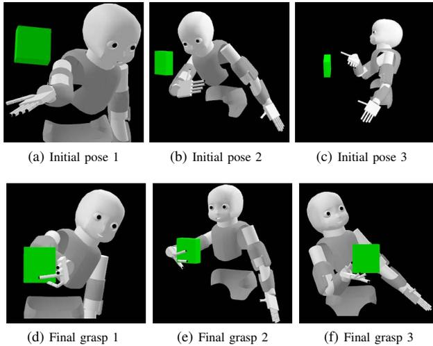
Fig. 5: Examples of iCub hand grasping of a cuboid. The first row (a,b,c) shows the initial postures and the second row (d,e,f) shows the corresponding final grasps.
